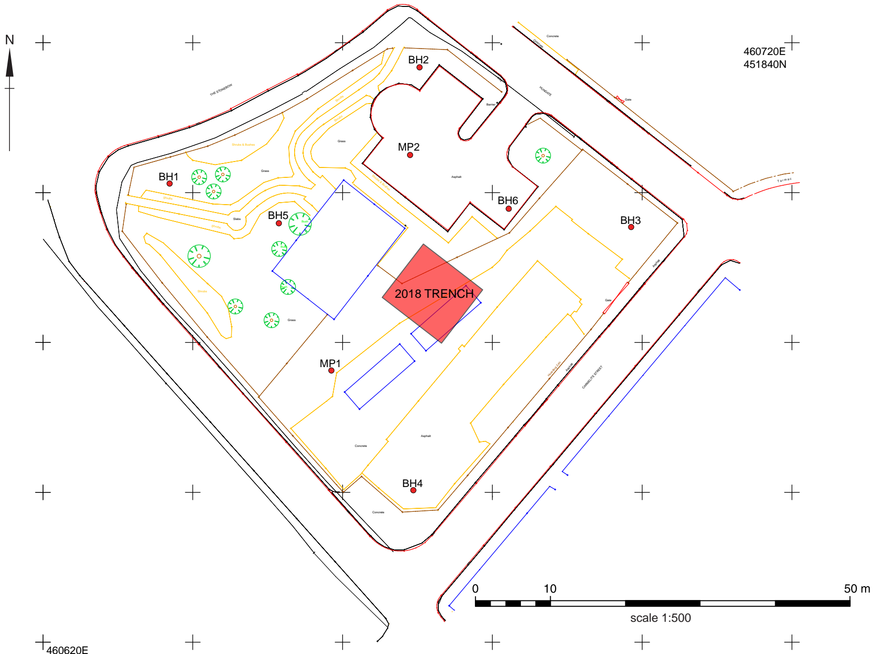
Fig. 3 2018 borehole and trench locations
