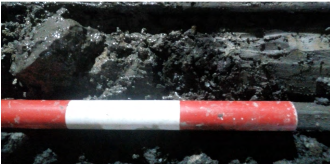
Plate 6 Borehole 3 organic deposit beneath cobbled road
