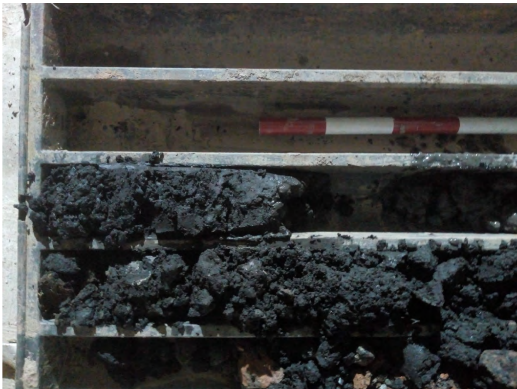
Plate 2 Borehole 1 Organic rich silty clays
