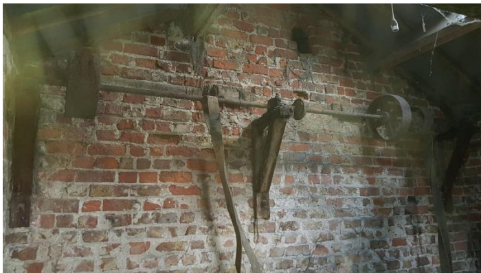
Figure 10: Cast Iron Drive Shaft with Flywheels and Attached Pulleys.
