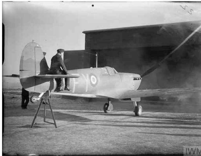
C) Spitfire firing at gun butts at Digby, Lincolnshire (source: ©Imperial War Museum photograph C 411).
