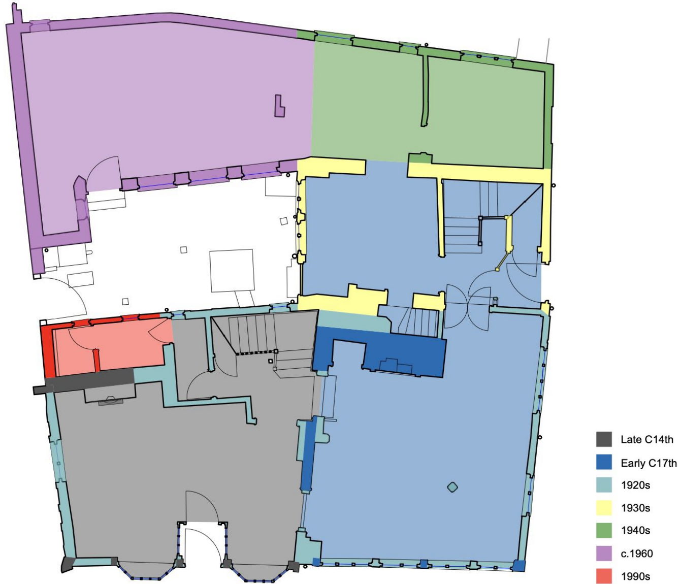
Figure 21 Phased Ground Floor Plan based on fabric analysis and documentary evidence. Block phasing shown paler; with specific identified historic fabric shown darker (not comprehensive).
