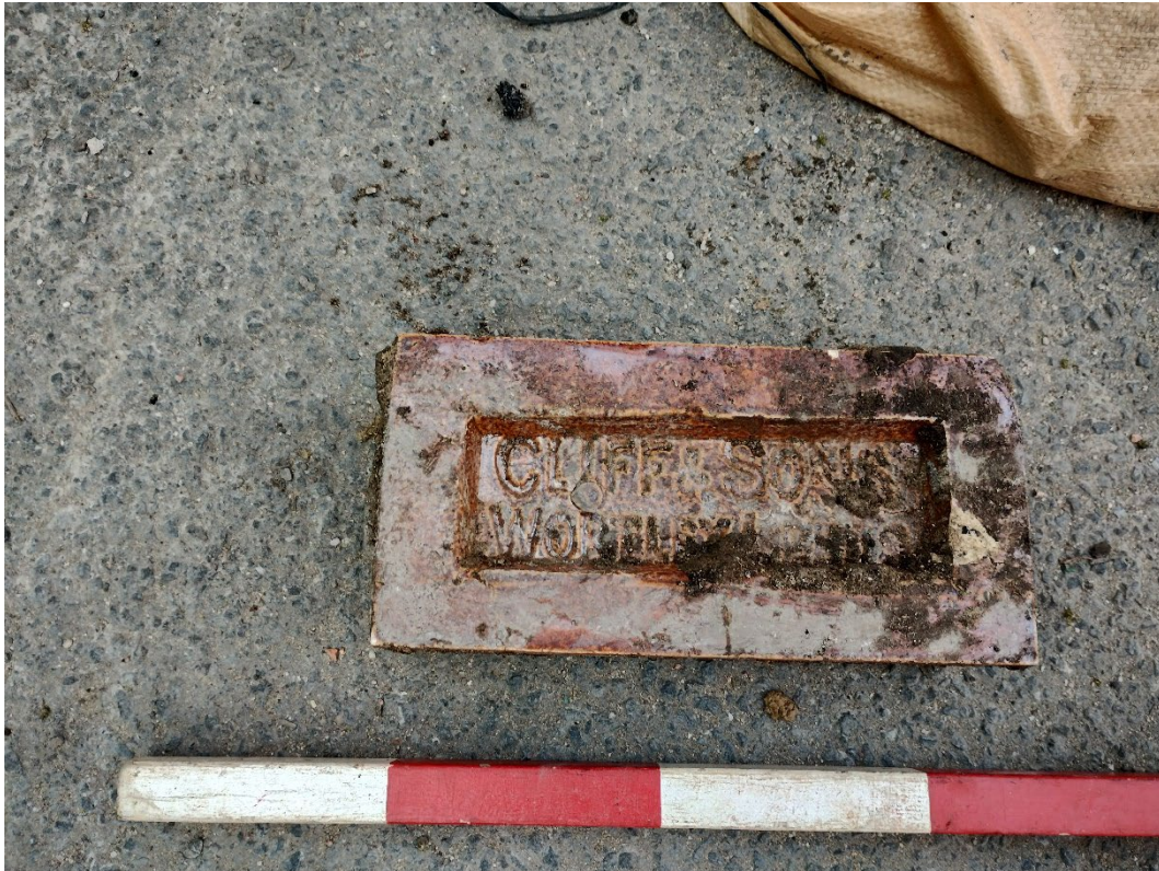
Plate 2: Brick displaying the brickmarker's mark: Cliff & Sons / Wortley-Leeds
