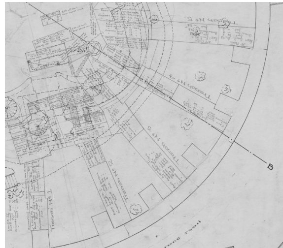
Plate 97 Mott drawing of underpinning locations, dated 1902
