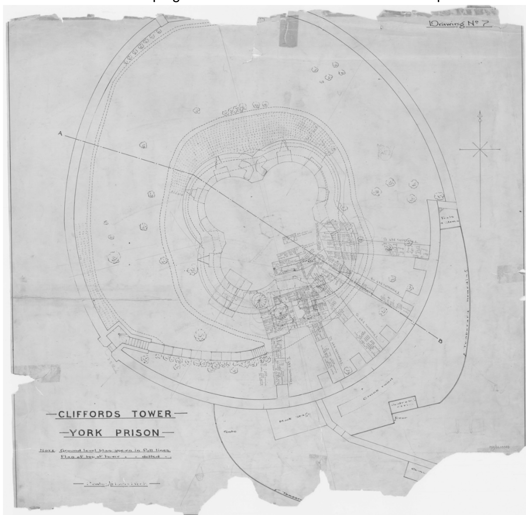
Plate 14 Plan of underpinning trenches (MP/CLI0003)
