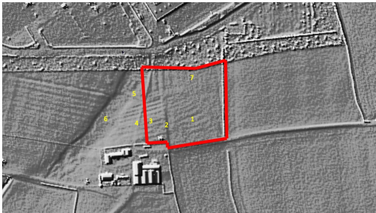
Figure 3: Features 1 to 7 observed during walkover survey; development site extent in red, lidar DTM background.
