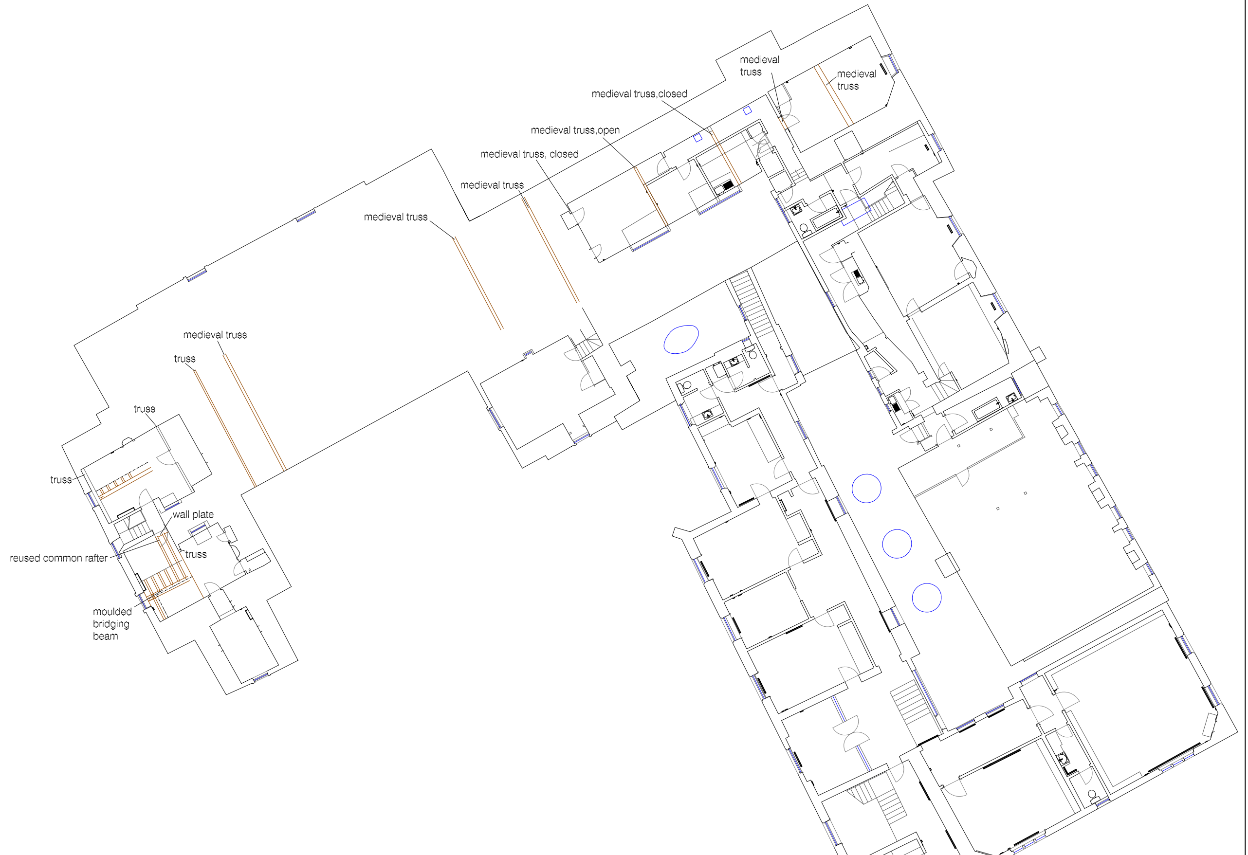
Intervention 5 - plan of in situ floor timbers and trusses at second-floor level, north range
