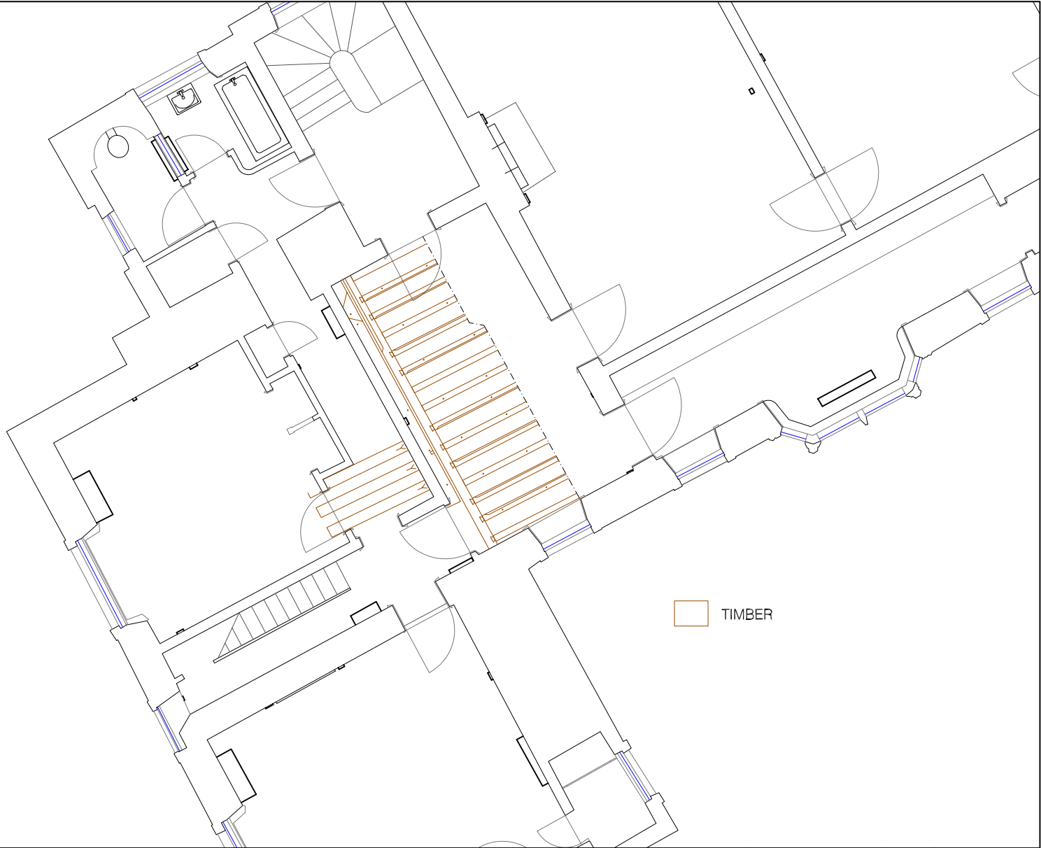
Intervention 5 - plan of re-used floor timbers at first floor level, southwestern half of the north range
