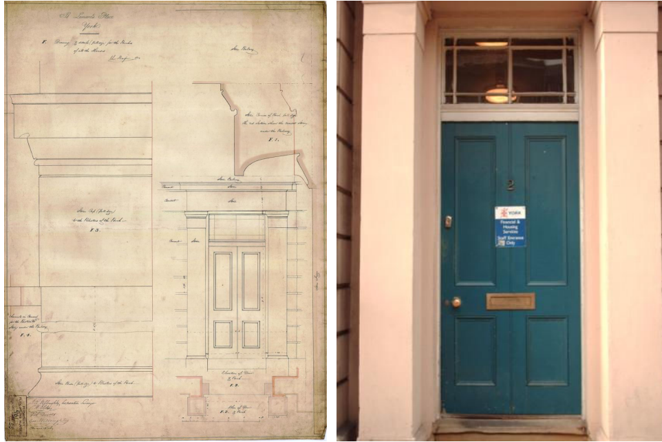
Figure*16A - Drawing & details (full size) for the Porches of all the Houses. John Harper 1834. (York City Archives, ACC 191/PH55/961)
